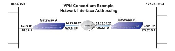
Figure C-4: VPN Consortium example network interface addressing
